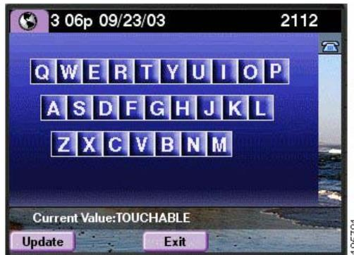
If the coordinates that are supplied in `<TouchArea>` tag exceed the dimensions of the phone display, the `<TouchArea>` rectangle will be “clipped” to fit. See Table 3-2, “Cisco Unified IP Phones Display Image Sizes and Color Depths” for a listing of usable display resolutions for each phone model.
